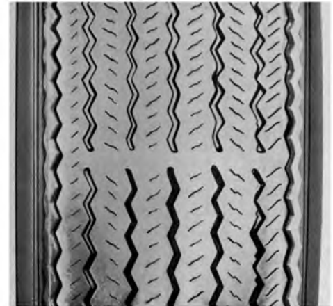
Indicator visible – tread worn
