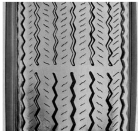
Indicator visible – tread worn
