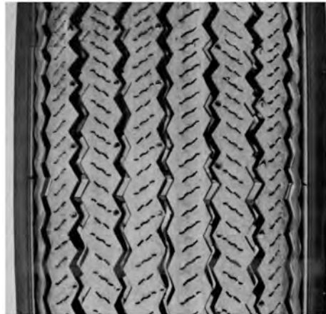
Tire in good condition
